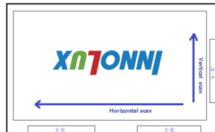
Fig. 2 Reverse scan (Pin24, Reverse = High)
